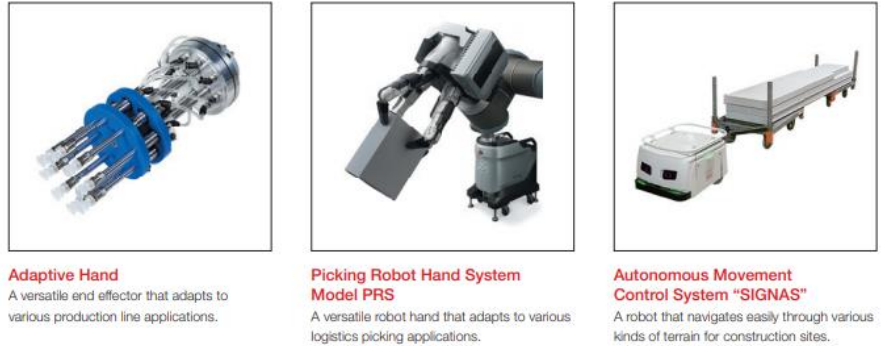
Figure 22: THK Co Ltd introduced these new automation products at the 2019 International Robot Exhibition
