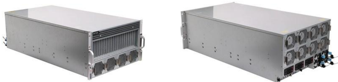
Figure 5: ZOTAC ZRS-326SV2 6U eight-GPU server platform
