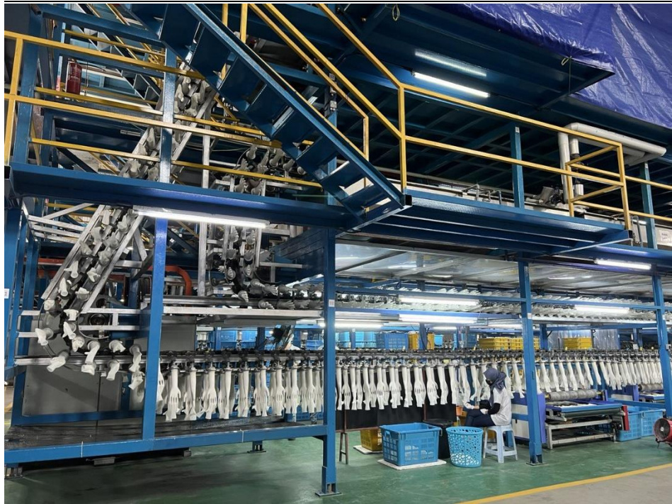
Figure 15: Glove production line, worker inspecting newly produced gloves for defects
