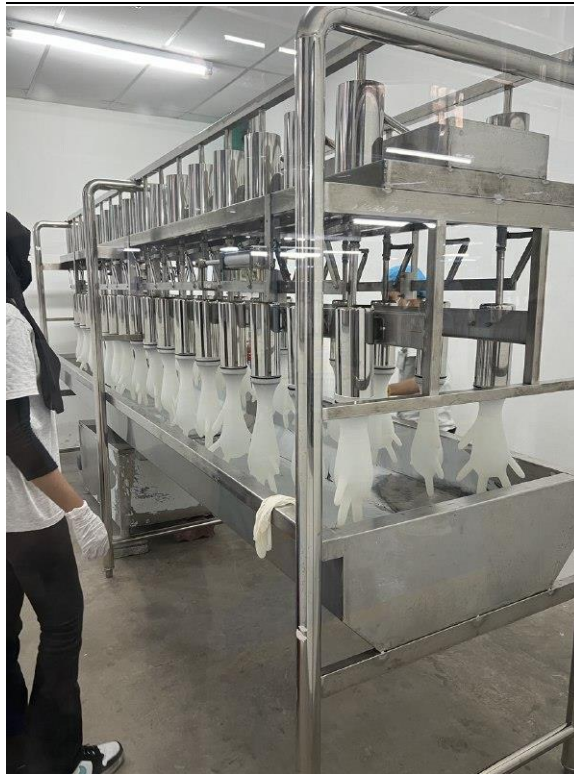
Figure 17: Checking for leakages in a batch of gloves
